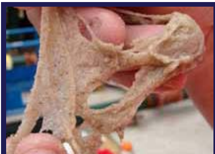
SlurrySMART Grouting Effect in Cohesionless Sands
